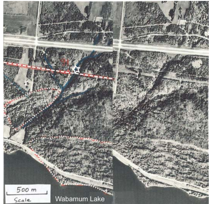
Figure 2 Top: Stereogram of pipeline (dashed) near Wabamun Lake, 90 km east of Edmonton, Alberta, showing large areas of landsliding along the shore of the lake (dotted). Star shows location of Figure 3.
