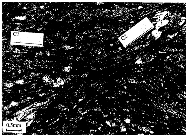
Figure 3. Photomicrograph of mylonite in domain 3 showing C1 and C2 foliations intersecting to give sinistral shear sense. Foliations are marked by acicular hornblende, epidote, chlorite and quartz grains. Plane light, north is to the top.
